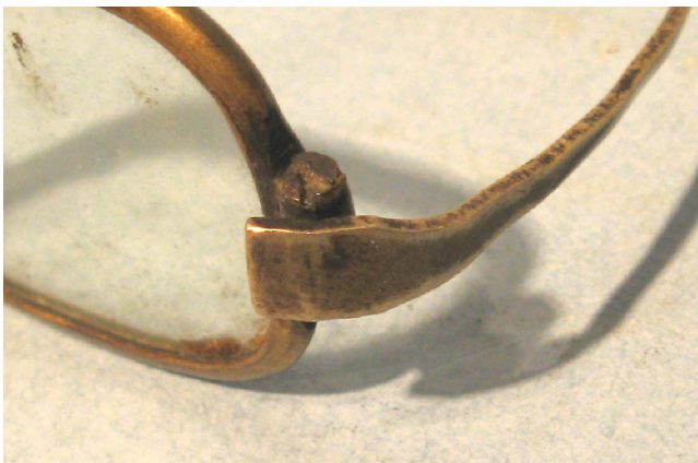
Close-up of the single pin joint found on inexpensive spectacles.
