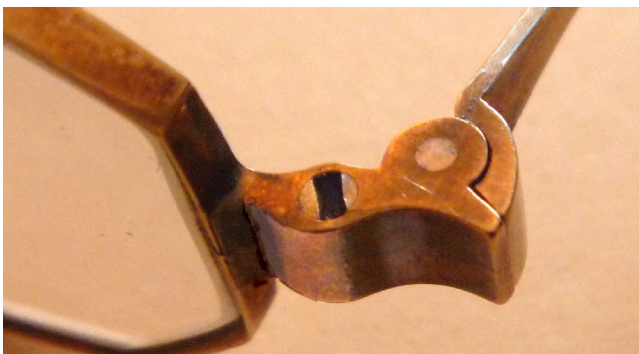
The most common type of spectacle joint, used for 150 years. A screw holds together the two halves of the joint. The temples are attached using a separate pin. This style of joint was used on silver, gold, steel, German silver and plated spectacles.
